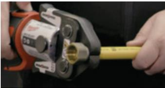
**5. USE THE HYDRAULIC PRESS TOOL TO FIX IN PLACE**
